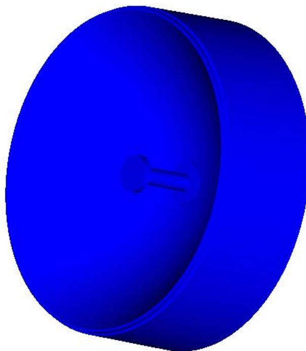
Figure 2. The reflector antenna with hat feed.
